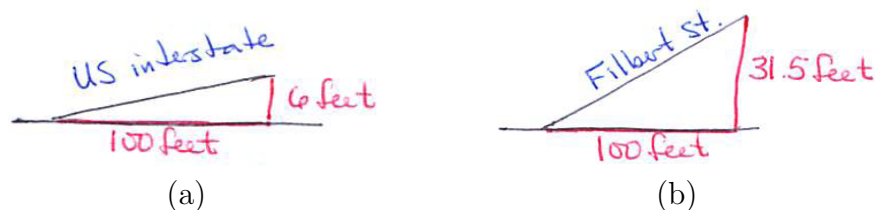
Figure 2.1.2: (a) Steepest US interstate has slope 0.06 and (b) Filbert Street has slope 0.315. [EDITOR: Replace with annotated pictures.]
