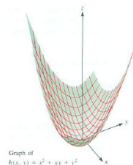
Graph of h(x, y) = x^2 + xy + y^2 Function has no global extrema Figure 16.6.4:
