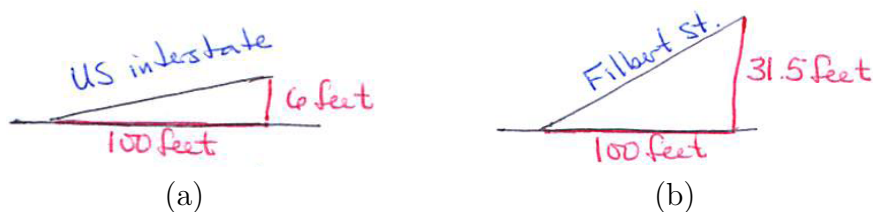
Figure 2.1.2 (a) Steepest US interstate has slope 0.06 and (b) Filbert Street has slope 0.315.
