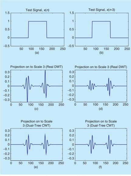
[FIG17] A signal x(n) and its shifted version x(n-3) (a), (b) and its reconstruction from wavelet coefficients at scale level 3 of the real DWT (c), (d) and dual-tree  $\mathbb{C}WT$  (e), (f). The  $\mathbb{C}WT$  is more nearly shift-invariant than the DWT.
