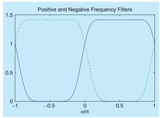
**[FIG4]** Hilbert transform FB. Magnitude frequency responses  $|H_p(e^{j\omega})|$  (solid) and  $|H_n(e^{j\omega})|$  (dashed) corresponding to (5).  $H_p(e^{j\omega})$  approximates  $H_a(\omega)$  in (63), while  $H_n(e^{j\omega})$  approximates  $H_a(-\omega)$ .
