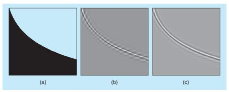
[FIG19] Near rotation invariance of the  $\mathbb{C}WT$ . (a) Test image with sharp edge on hyperbolic trajectory. (b) When the test image is reconstructed from one level of the DWT coefficients, ringing and aliasing effects are apparent. (c) The reconstruction of the image from one level of the  $\mathbb{C}WT$  does not exhibit these phenomena.
