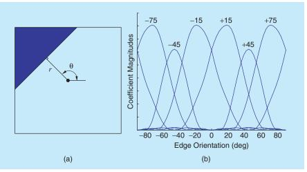
[FIG21] (a) Image segment with an edge singularity at orientation  $\theta$  and offset from center r. (b) Magnitude responses of the  $\mathbb{C}WT$  coefficients of this segment as a funtion of  $\theta$ .
