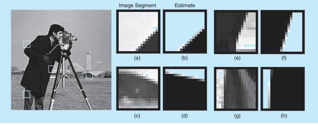
[FIG22] At top the Camerman test image and four segments with strong edges. Below, zooms of the segments plus idealized edges formed with the parameters estimated from the CWT magnitude and phase. (No attempt is made to match the texture within the segment, only the edge parameters.)
