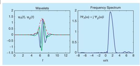
[FIG3] A q-shift complex wavelet corresponding to a set of orthonormal dual-tree filters of length 14 [58].
