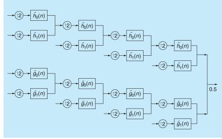
[FIG8] Synthesis FB for the dual-tree CWT.
